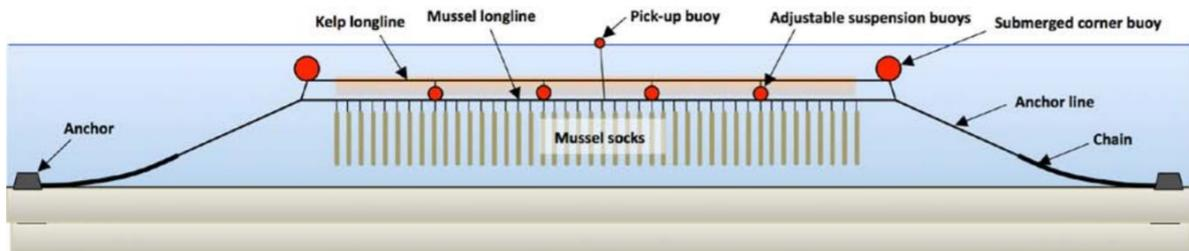
Figure 6: The double-headrope longline design (Lindell, 2016)
