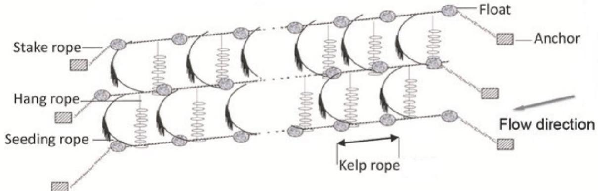
Figure 4: Example of a setup for combining rope culture and seaweed culture in China (Mao, et al., 2018)
