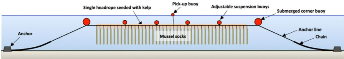
Figure 5: The dual-use single headrope system design (Lindell, 2016)
